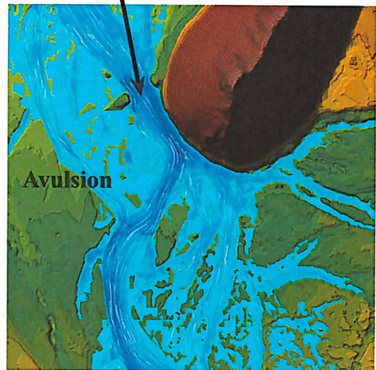
A HEC-RAS 2D model was used to simulate pre- and post-project flood conditions and demonstrate that 100 year flood elevation was unaffected by the project.
