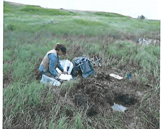
Soil pits are used to evaluate hydrology and hydric soil conditions.
