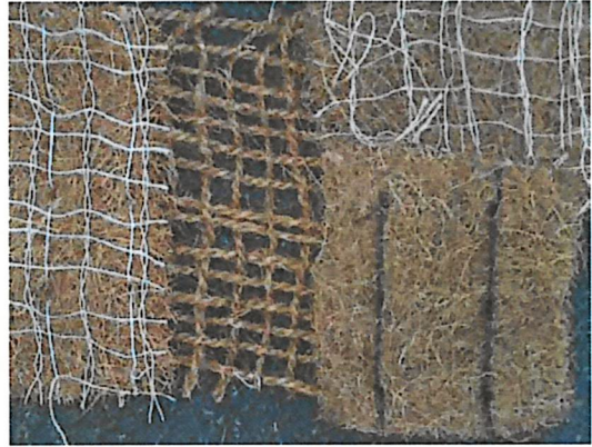
Natural fiber erosion fabrics are commonly made with coconut or jute.
