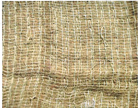
Finer coconut fabrics are frequently layered beneath the coarse coir fabric to prevent loss of fine soils.
