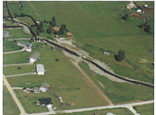
Aggrading “filling” channels result from excess sediment supply or reduced transport capacity.
