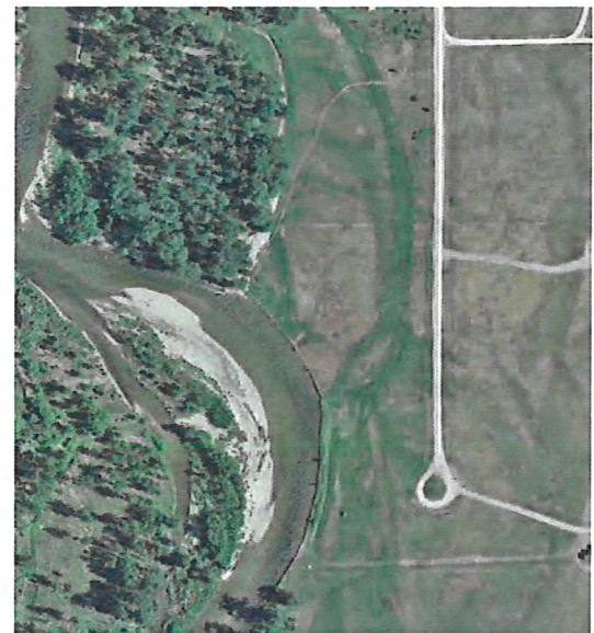
By 2015, the meander had encroached into the hayfield and floodplain. Is this a localized response to a lack of woody vegetation, a reach scale response, or larger adjustment process in the watershed?
