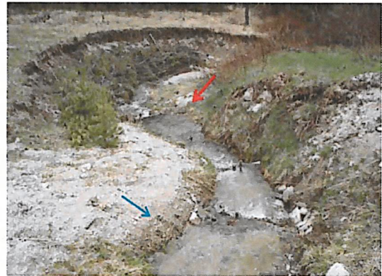
Incised channels are associated with stream channel downcutting and loss of floodplain connectivity.
