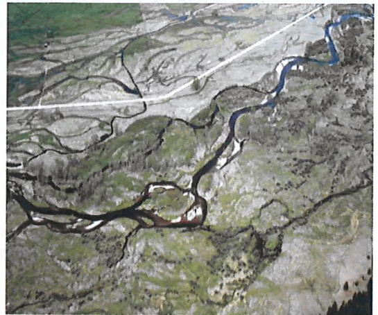
Degraded C4 (wide, shallow channel) trending to D4 (multiple thread, unstable form). This channel could recover through riparian management to promote woody vegetation.
