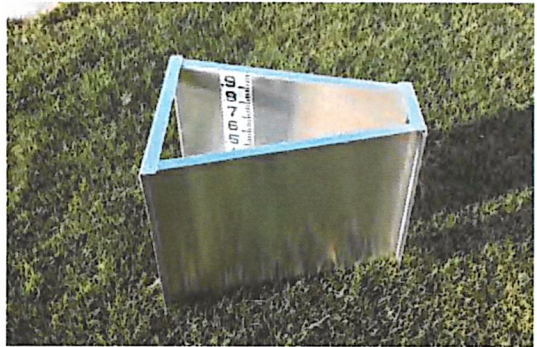
The Montana flume is a shortened version of the Parshall and must be free flowing (not backwatered).
