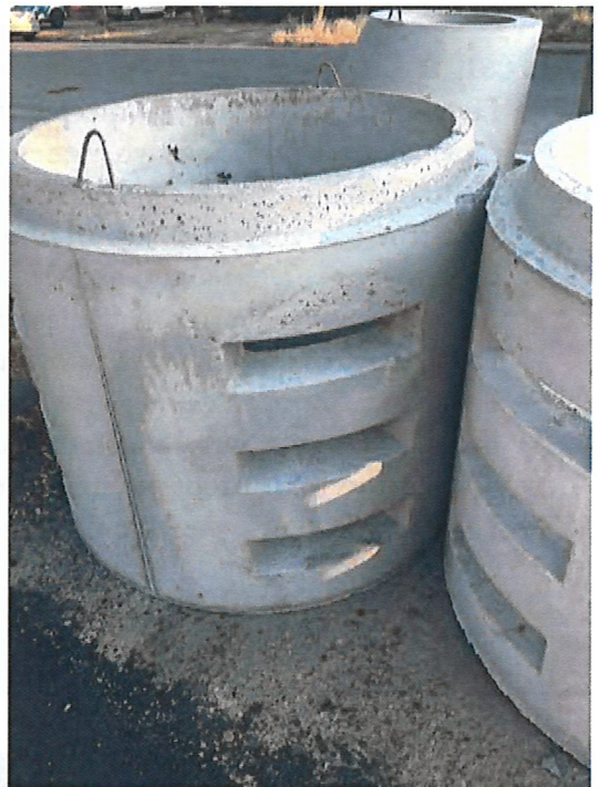
Concrete rings can make excellent pumping vaults when buried adjacent to a gravel bed stream channel.
