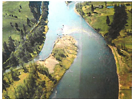
Berms can direct flow against the opposite bank and cause erosion on the other side of the river.
