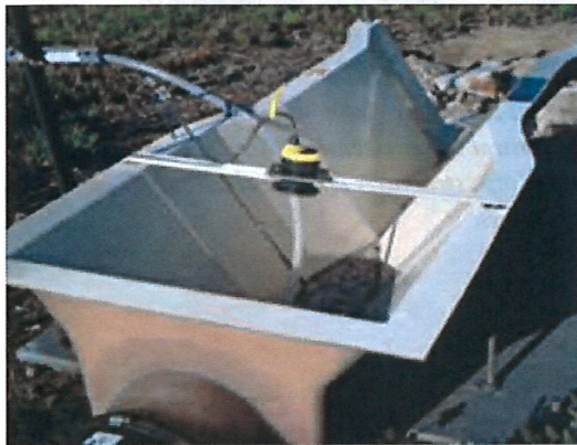
Numerous commercial water level/telemetry systems are available to measure flow remotely, including ultra-sonic and other sensors.
