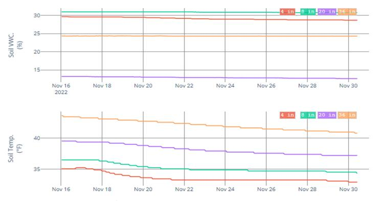
Soil moisture and temperature data for the Manhattan probe on November 30th 2022 is shown in the above table and graphs. See next page for the Bozeman probe information for November 30th 2022 and soil moisture summary data.
